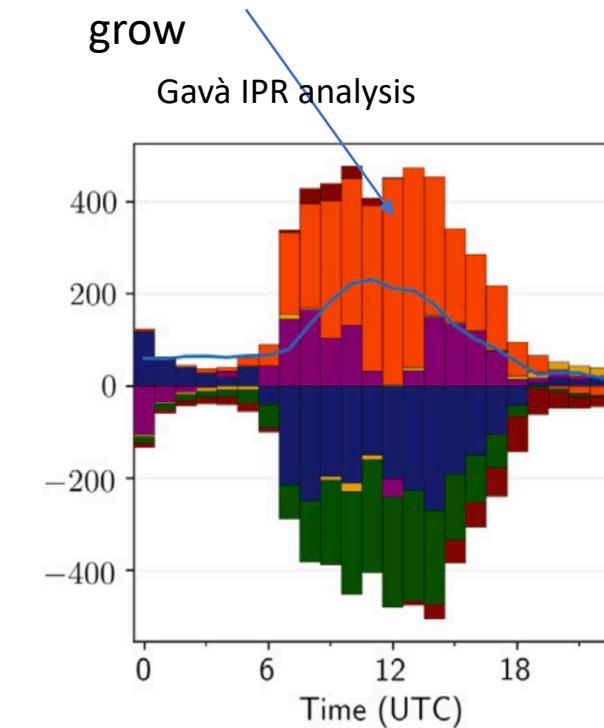
Process analysis shows vertical diffusion in a coastal station -> ozone fumigation (Jaén et al 2021)
